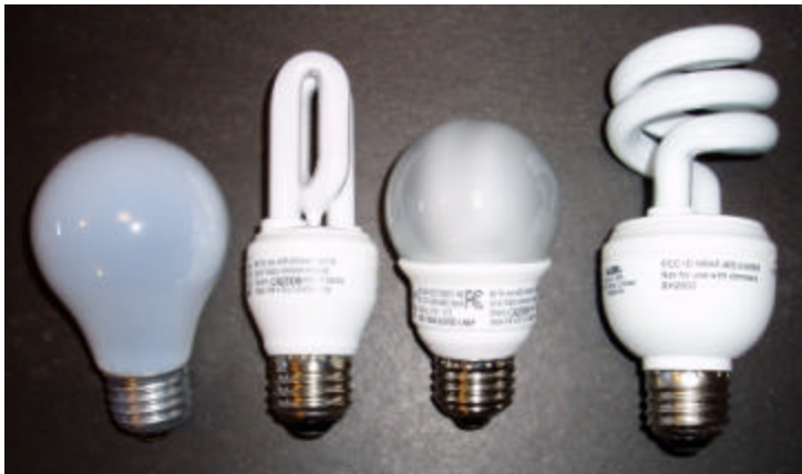
Compact fluorescent lamps (CF lamps) last longer and are cheaper to operate than regular light bulbs. A typical 15 Watt CF lamp is as bright as a standard 60 Watt incandescent.
