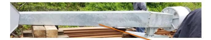
Tail boom incorrectly installed upside down
