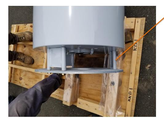
NOTE: The clamp plate spacers are from a previous revision. Current production will have hardware to mount the nose cone already installed
