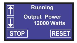
In normal operation the Powersync II will show the status as "Running" and will display the instantaneous Output Power in Watts. Other operating modes that may be indicated are as follows:
