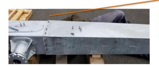
WARNING: The tailboom bolts must be installed with hand tools. Using an impact driver WILL damage the nuts.
